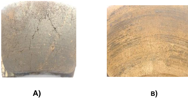
FIGURE 11 : FLOATING SURFACES OF LININGS AFTER PERFORMANCE TEST: A) UF10-50-0.2 LINING; B) COMMERCIALY AVAILABLE LINING
